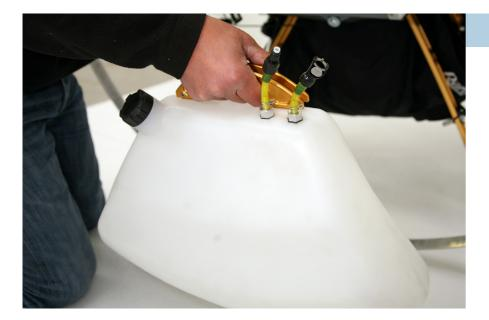
Insert the fuel tank - The bottom of the tank will engage with the dowels on the lower frame spars.
